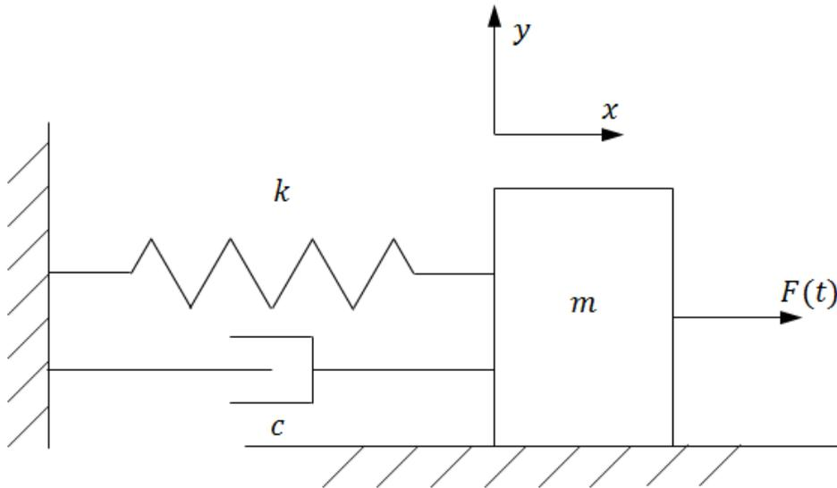
Fig 1: Spring-mass-damper with external force
